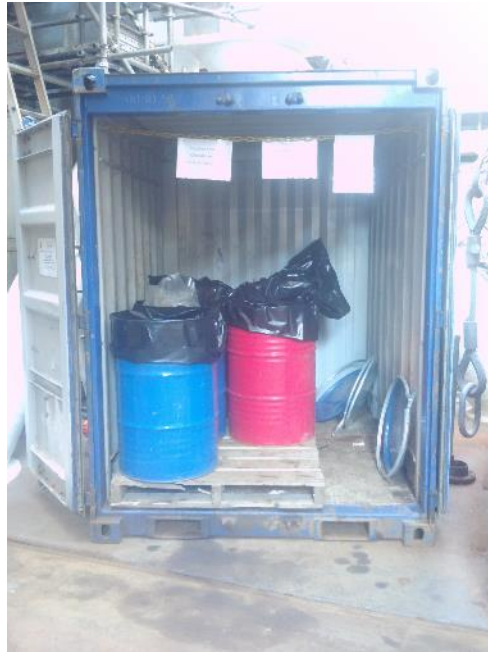
Photo 11. Container for storage of drums for oily rags (when full, entire container will be transferred to shore)
